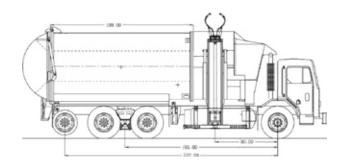
**BODY CONSTRUCTION** Body Shell - 1/8" Hardox 450
